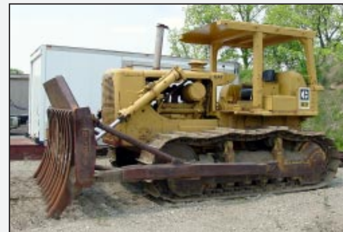
Caterpillar D7F Dozer, will have Straight Blade installed.
